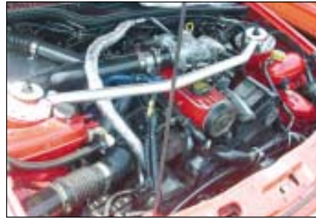
Larry Davis: Ported head, big valves, gutted upper intake, knife-edged lower, air-to-water I/C, Ranger cam, K&N, SDS fuel and ignition management system, 52 lb./hr. injectors.
