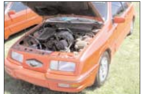
Dejan Cokic: His red '89 sports a home-made Cossie-style grille for increased underhood cooling, and a TurboCoupe inter-cooler.
